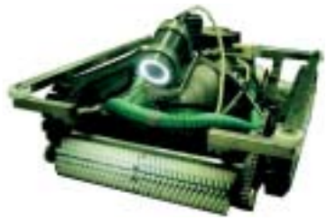
Weda's robot with the Mariner underwater camera fitted.
